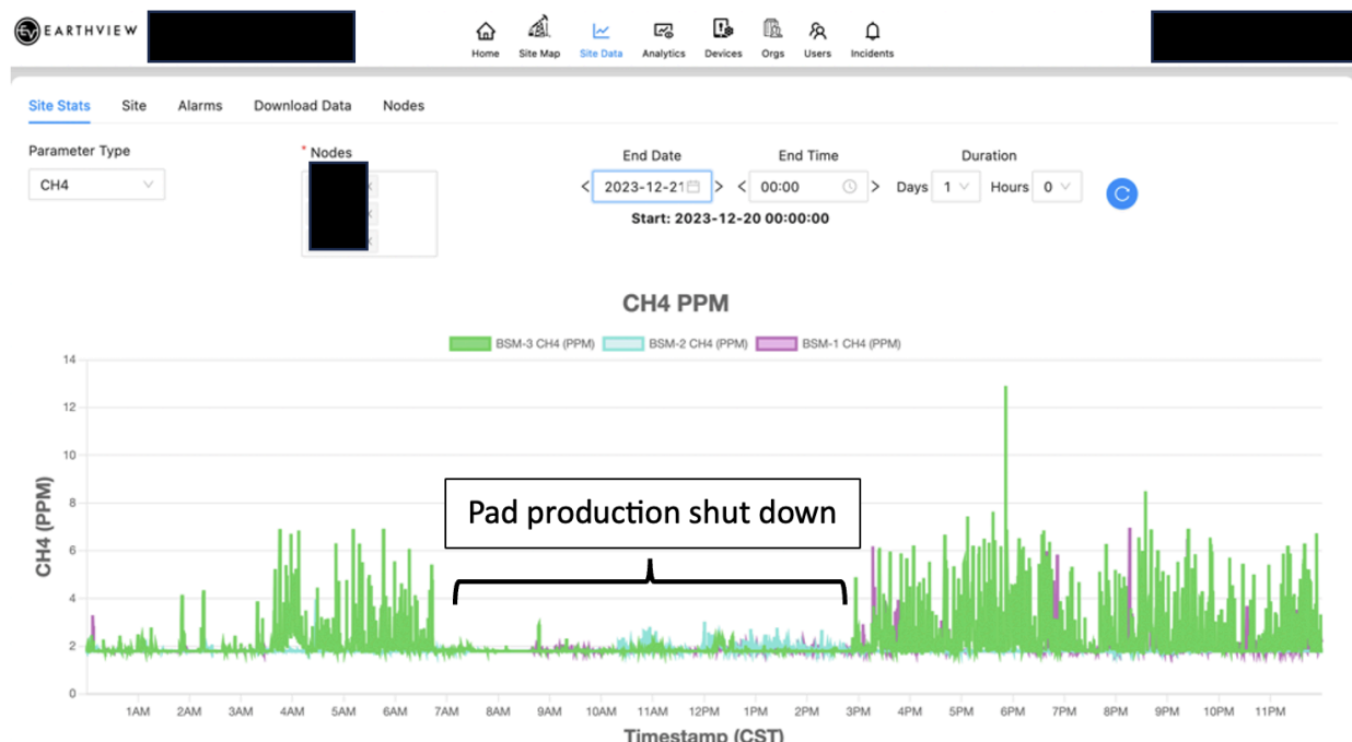
Figure 31. Detection of emission differences between background pad operations and a pad shut-down period. The x axis is time in UTC. The y axis is CH4 concentration in ppm.
