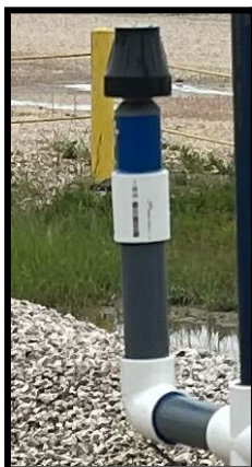
Figure 4. Communication Antenna. Sends local measurements to Earthview cloud servers.
