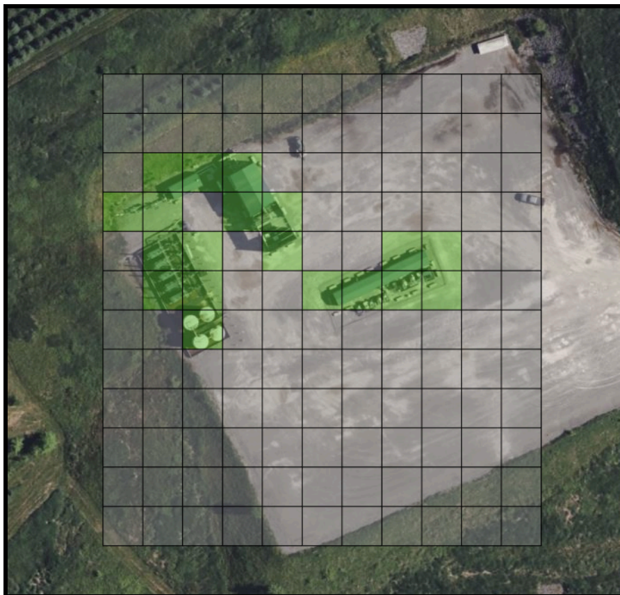
Figure 17: Grid layout over potential leak locations. Green cells indicate a potential leak location, gray cells indicate locations without any known equipment.
