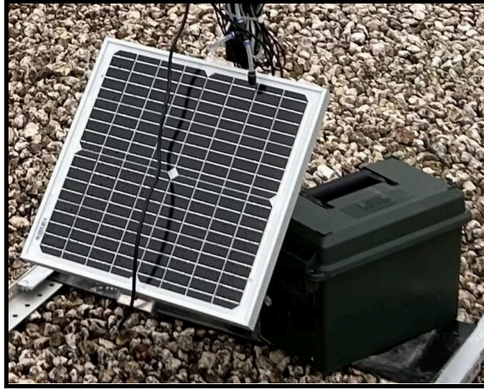
Figure 5: BluBird power supply system: solar panel and backup battery.
