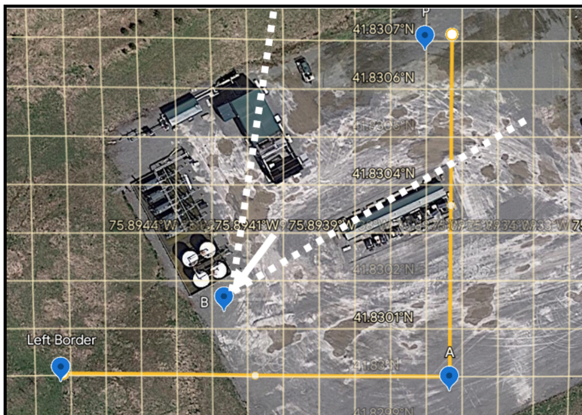
Figure 16. Sensor cone of visibility. Each sensor (blue pin) has a 70° “cone of visibility” (dotted white line) that opens into the current wind direction (white arrow).
